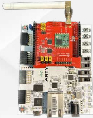
Figure: Arty-a7 100T FPGA with SX1276 based LoRa shield
