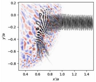
Wave propagation in turbulent plasma in presence of sheared flow Example of the coupling of the fullwave code with GYSELA simulation (from S. Rienäcker) References : [Burrel, Physics of Plasmas 27, 060501 (2020)]
