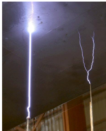
Photography of 2.5 m long discharge guided by laser filamentation (left one).
