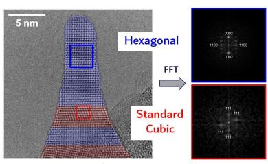
Plasma source in operation and atomic-resolution view of a hexagonal silicon nanowire grown *in situ* in NanoMAX.
